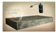
Cleaning with a jet of water, penetration of remainders (acids, parasites, and other biological waste) by the cracks and pores in the capillary network of the concrete.
